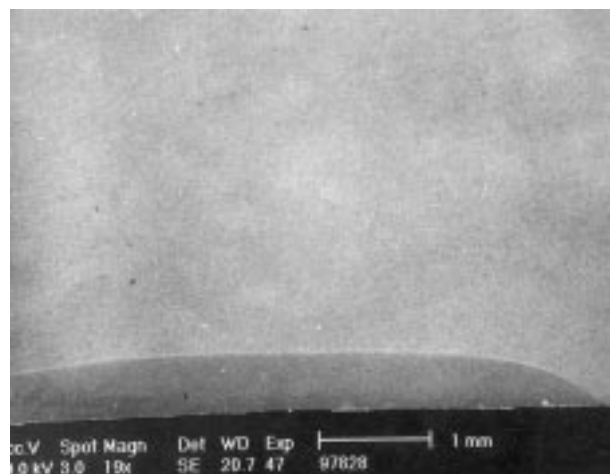
Fig. 2 A full view of the quenched zone near the outside corner of the groove. (Art has been enlarged to 133% of its original size for printing.)
